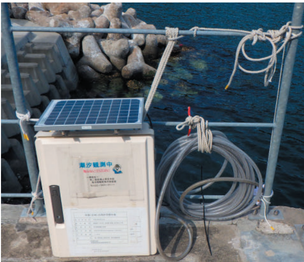
Photo 5. Hydraulic-type installed outside the Kamaishi tide station.
