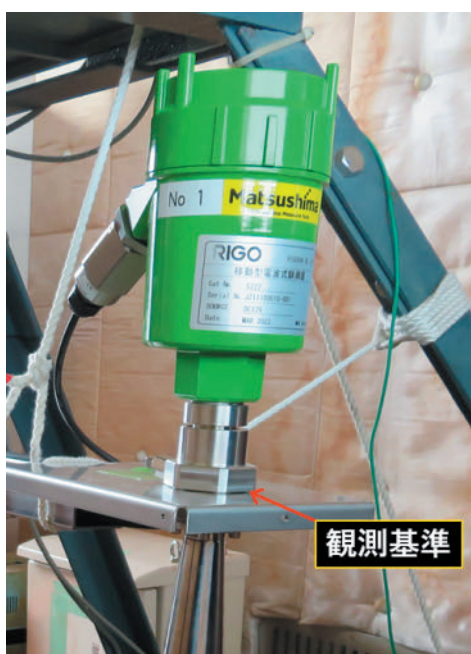
Photo 3. Observation standard of portable radio wave-type (0th place).
