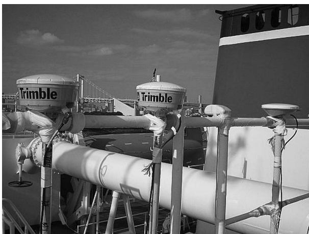
第3図 測量船「昭洋」のGPSアンテナ設置状況 (右からKGPS, MSAS, DGPS) Fig. 3 Arrangement of installation of GPS antennas on survey vessel "Shoyo" (for KGPS, MSAS, DGPS from the right).
