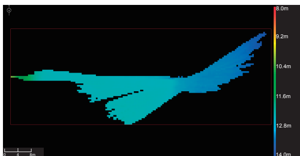
Fig. 7. 0.5 m gridded reference bathymetric data of stationary observation (phase A-2) obtained with SeaBat 8125.
